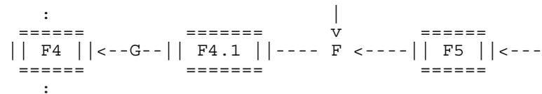
F4.1 = Sensor Instrument. Translates the sensed variable F into some kind of a reading or metric. A pressure sensor turns a pressure into a voltage. Sometimes combines some set of physical sensors into a reading or set of readings. Note that I may measure the temperature of a vessel and translate it into the temperature of the substance inside the vessel. Sometimes samples or averages a continuous reading.
