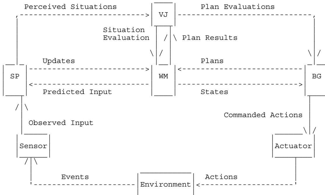
The system portion of this busy looking elemental loop repeats in a hierarchical manner, much as the elemental loop in PCT repeats in a hierarchy.
