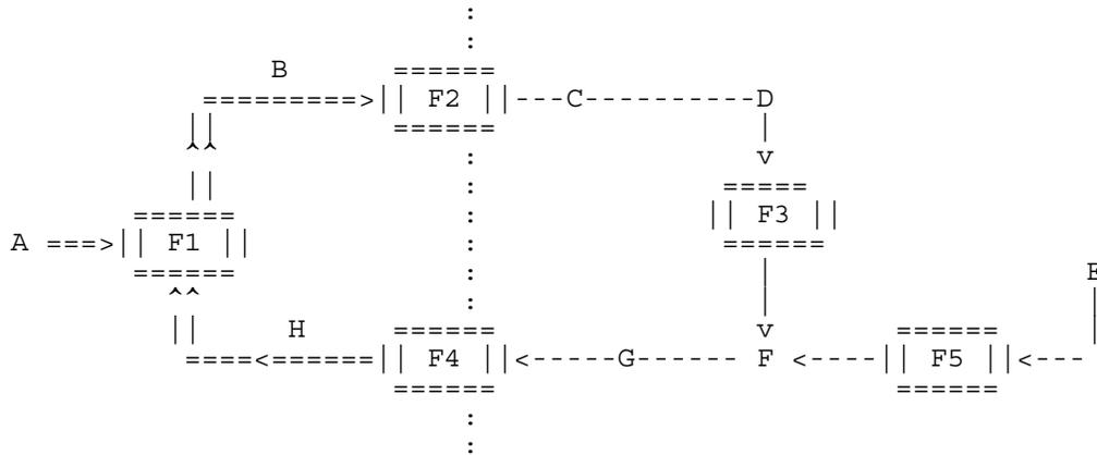
The vertical dotted line separates the control system (to the left) from the physical (observable) environment outside it (to the right).
